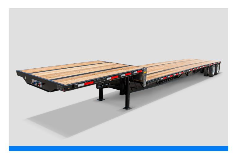
The Wabash Steel Drop Deck Platform is built to last. Heat-treated 130ksi steel provides high strength and low trailer weight. In addition, the premium paint process ensures best-in-class corrosion resistance and keeps your trailer looking good year after year.
