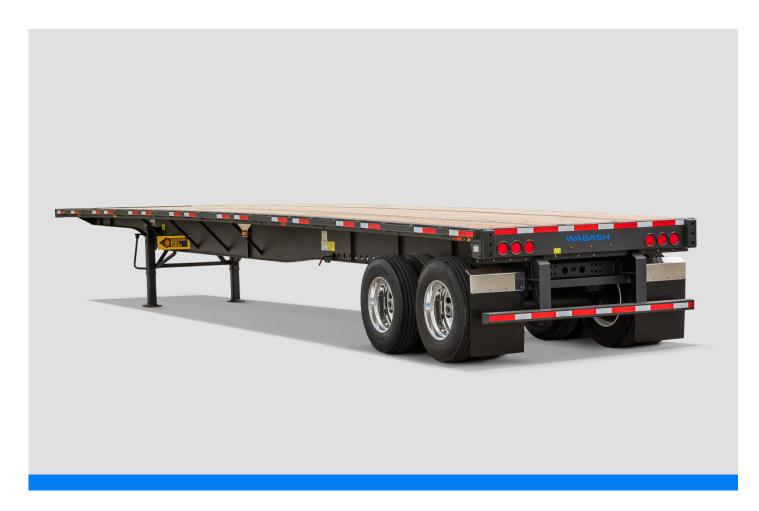
The Wabash Steel Flatbed is built to last. Heat-treated, 130ksi steel provides high strength and low trailer weight. In addition, the premium paint process ensures best-inclass corrosion resistance and keeps your trailer looking good year after year.
